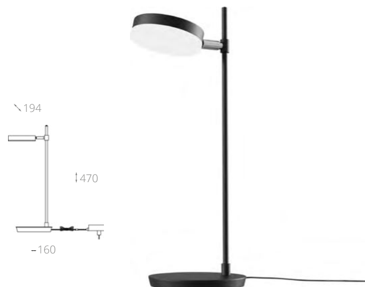
▲ MOD070TL-L8B3K LED 8W 450 lm, 3000 K, >80 Ra, 120 220-240 V, IP20 470 × 160 × 191 mm
